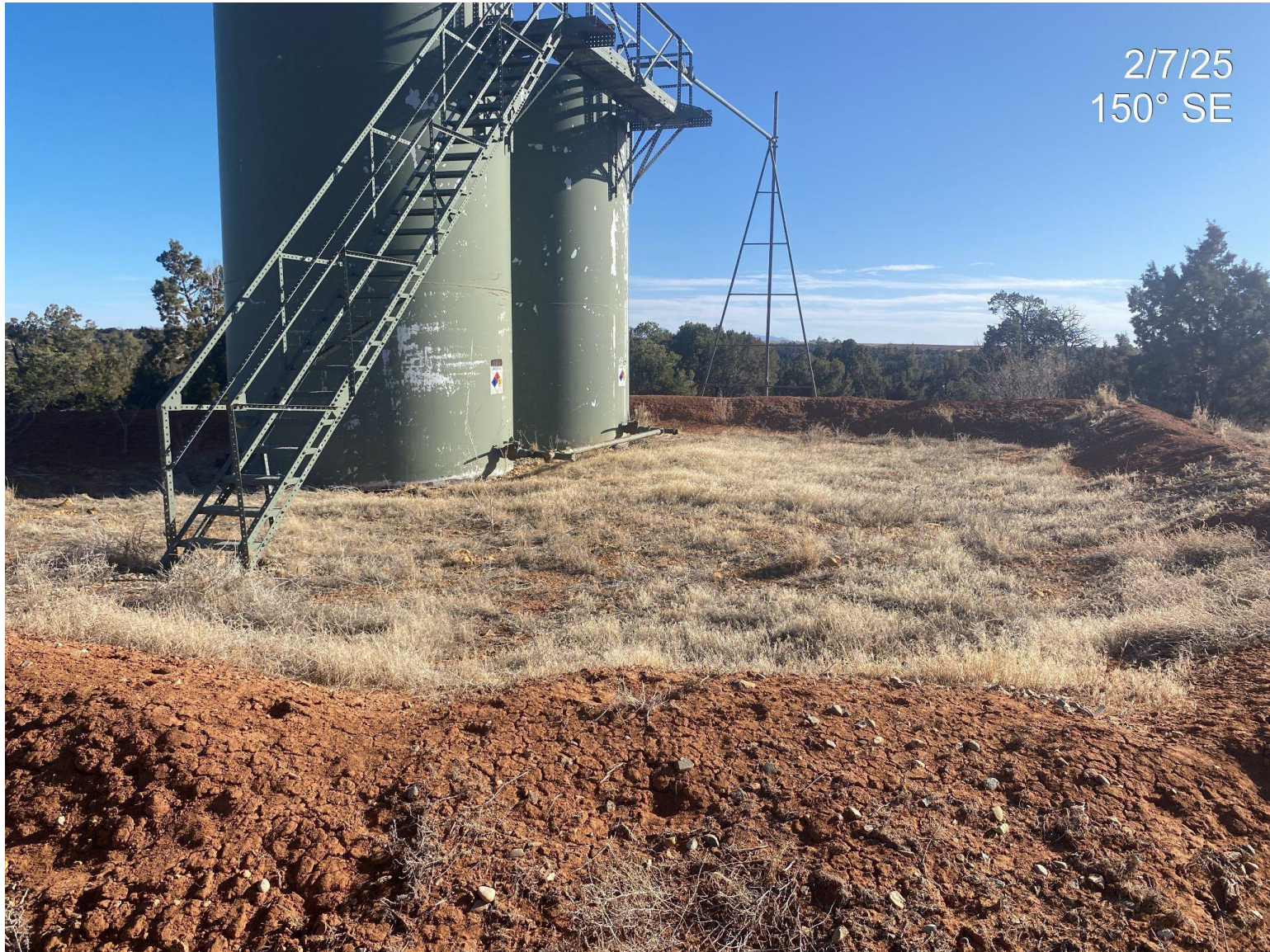
Photo 3. Vegetation/cheatgrass not maintained around equipment and within tank berms.
