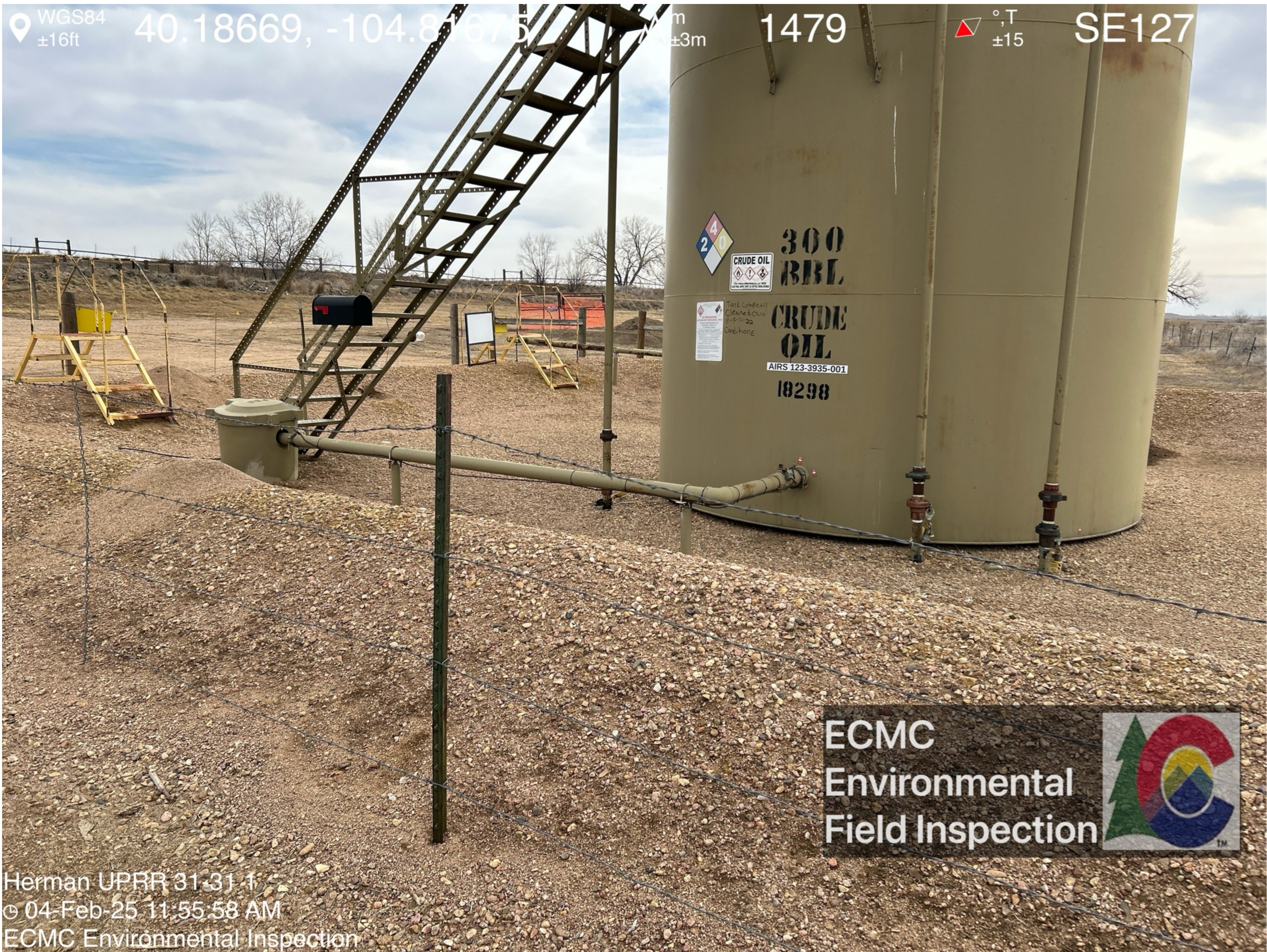
NFPA placard visible on production tank.
