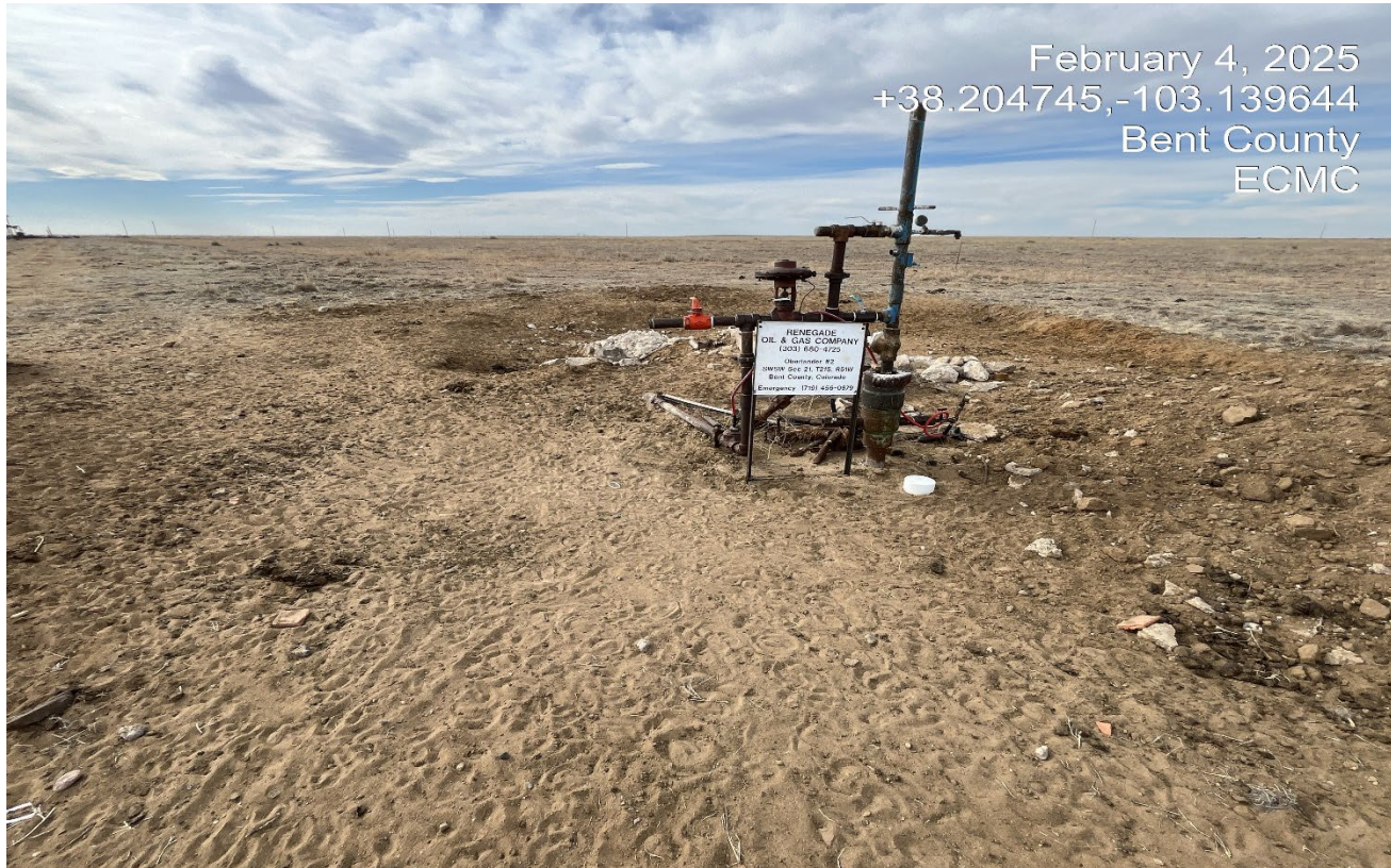
Photo 4. Facing toward the wellhead. There was a hissing gas leak heard at this well. The Operator was immediately notified. The emergency number list was disconnected.
