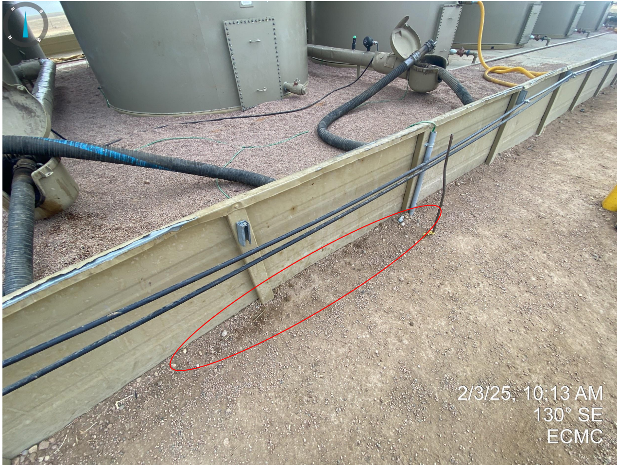
Photo 21. Stained soil observed near loadout lines, outside of secondary containment.
