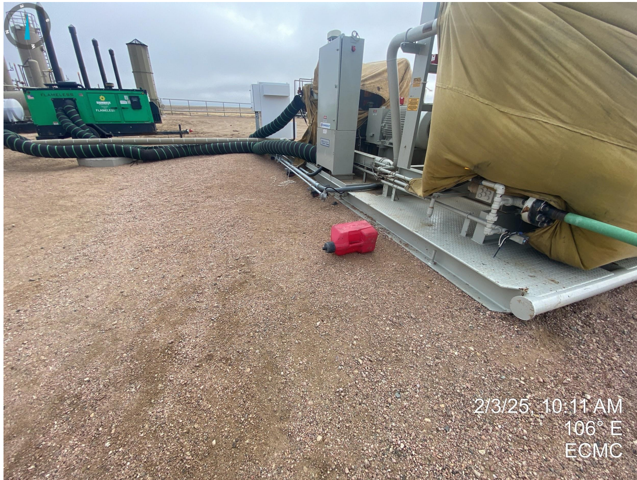
Photo 13. Gas can outside of secondary containment, near compressor.
