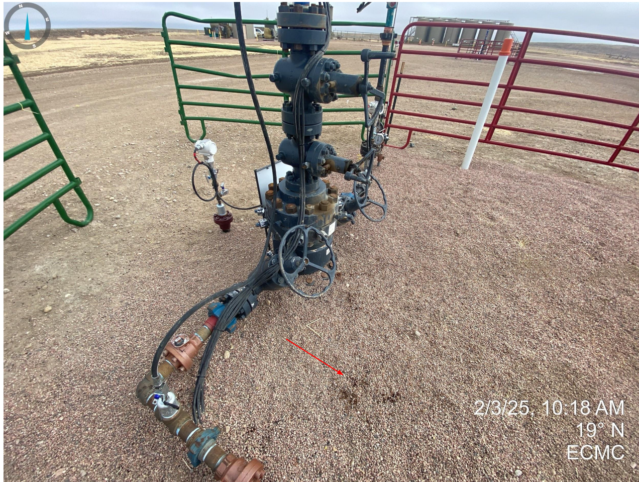
Photo 29. Stained soils observed at API #123- 50750.
