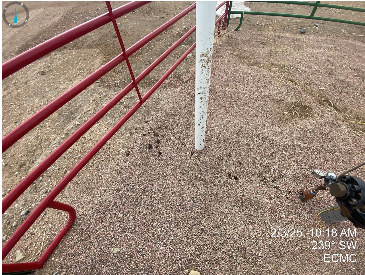
Photo 28. Continued from Photo 27; hydrocarbon staining observed near well head.
