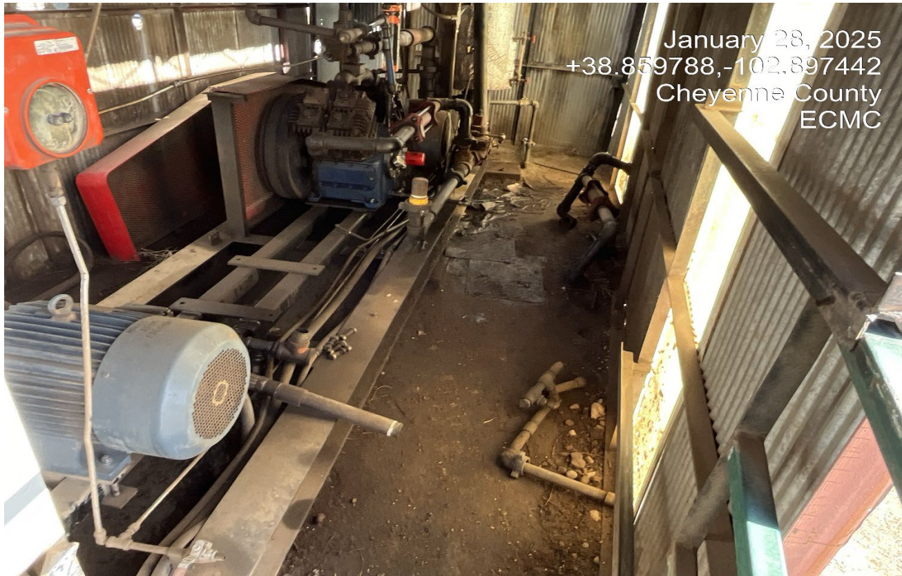
Photo 3. There is oil stained soils inside the shed from the leaking pumpjack engine.
