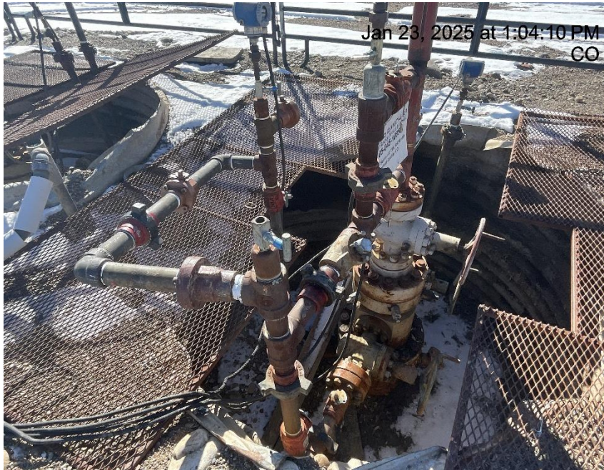
Photo # 1144 Cellar not properly covered/wildlife & personnel hazard
