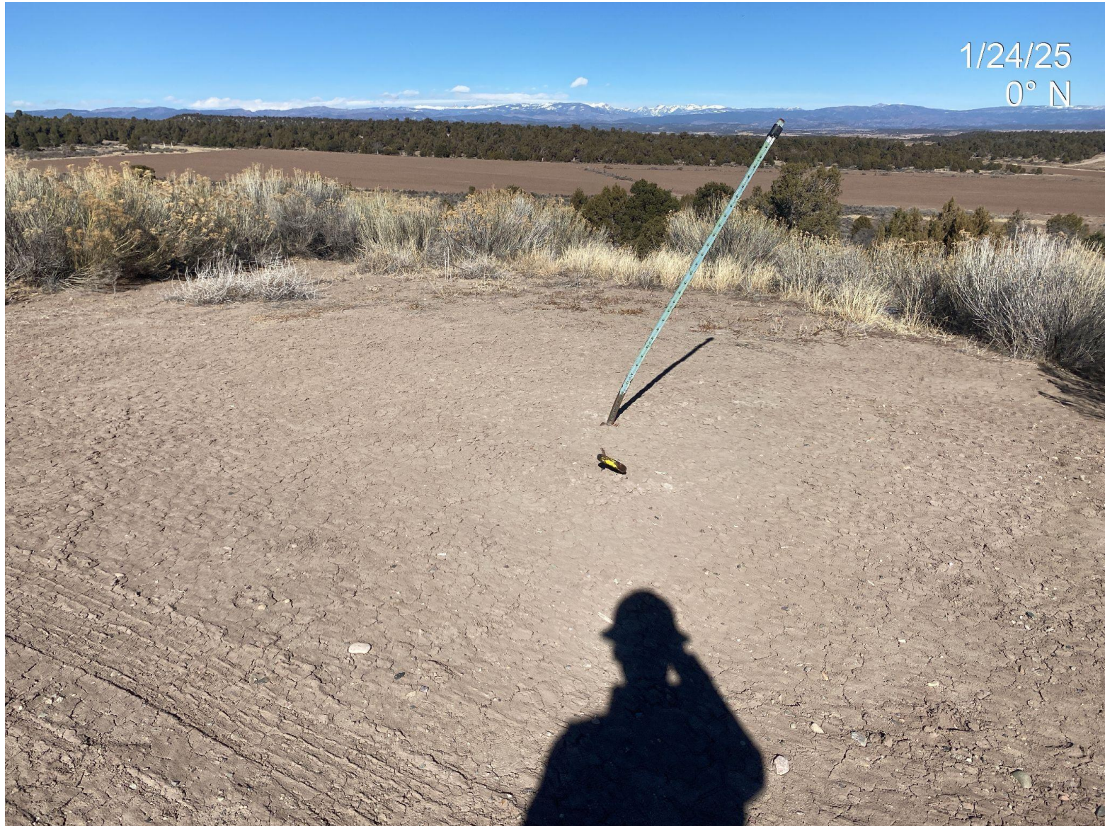
Photo 2. Marked guyline anchor.
