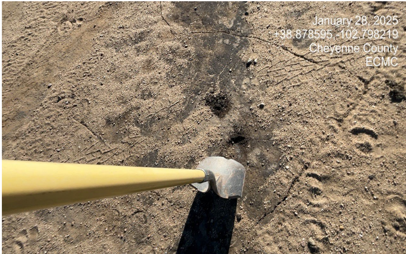
Photo 7. View of black hardened material shown at previous photo. All impacted soils must be cleaned up and removed.
