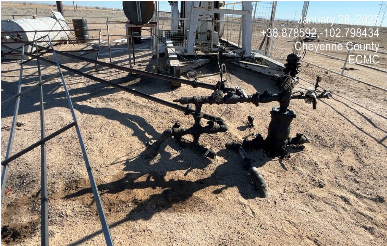
Photo 5. There is still stained soils around the wellhead from a E&P waste spill. It appears there was sand spread on top of the spill which was not cleaned up per the rules. Previous corrective action was not completed.
