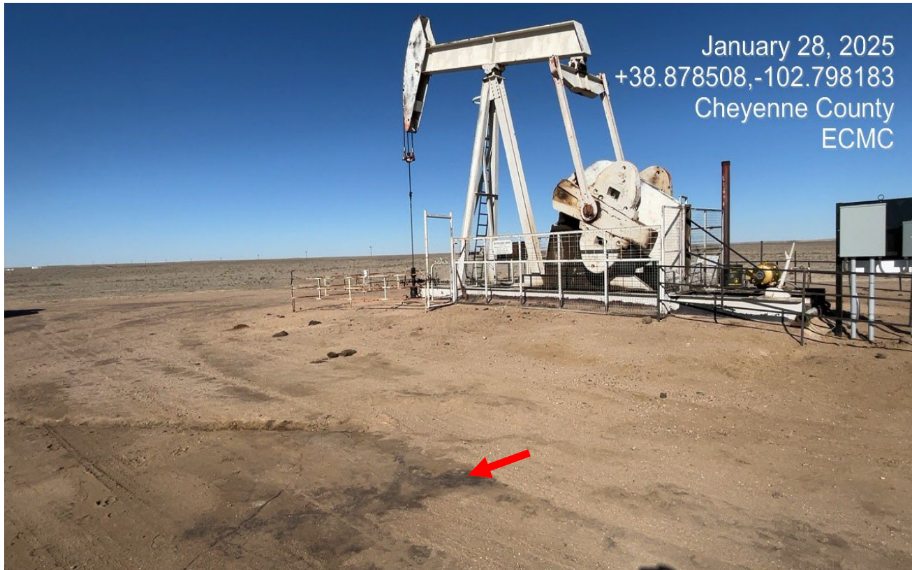
Photo 9. South side of the pumpjack facing northwest. There is black stained soil shown at red arrow.
