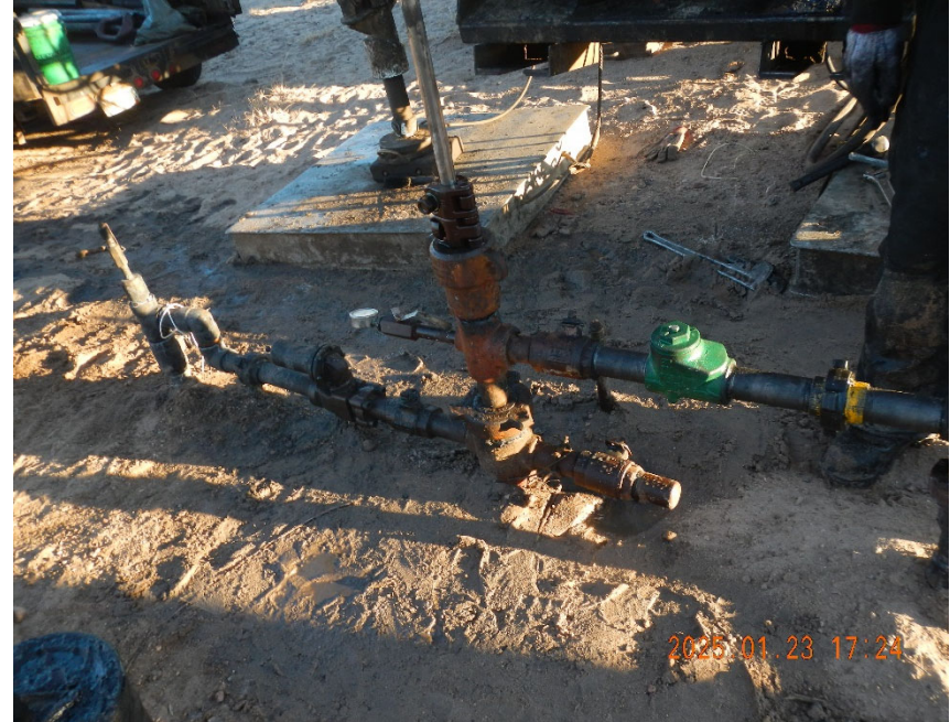
2. View of wellhead. Rods and Tubing are back in wellbore.
