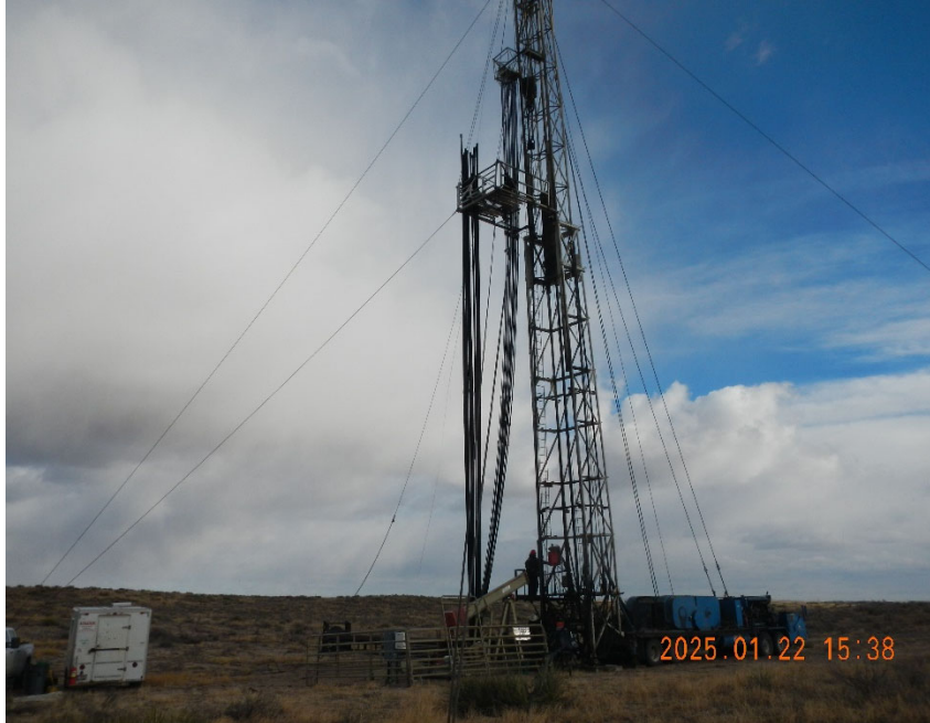
3. View of rig with rod string and tubing string in the derrick.
