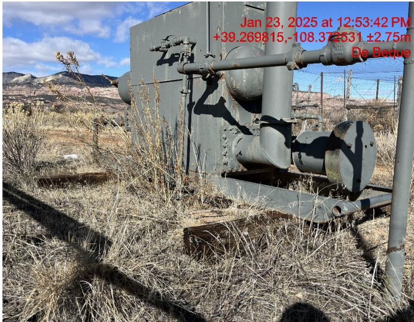
Photo # 3275 Weeds/undesirable plant species near production equipment causing a fire hazard
