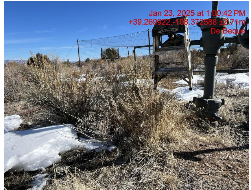
Photo # 3284 Weeds/undesirable plant species near production equipment causing a fire hazard
