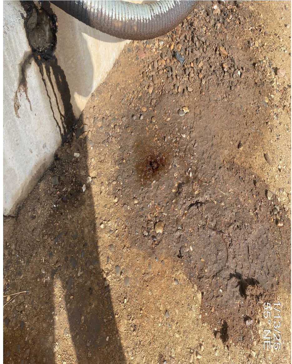
Photo 3. View of stained soils at the pump jack/muffler.
