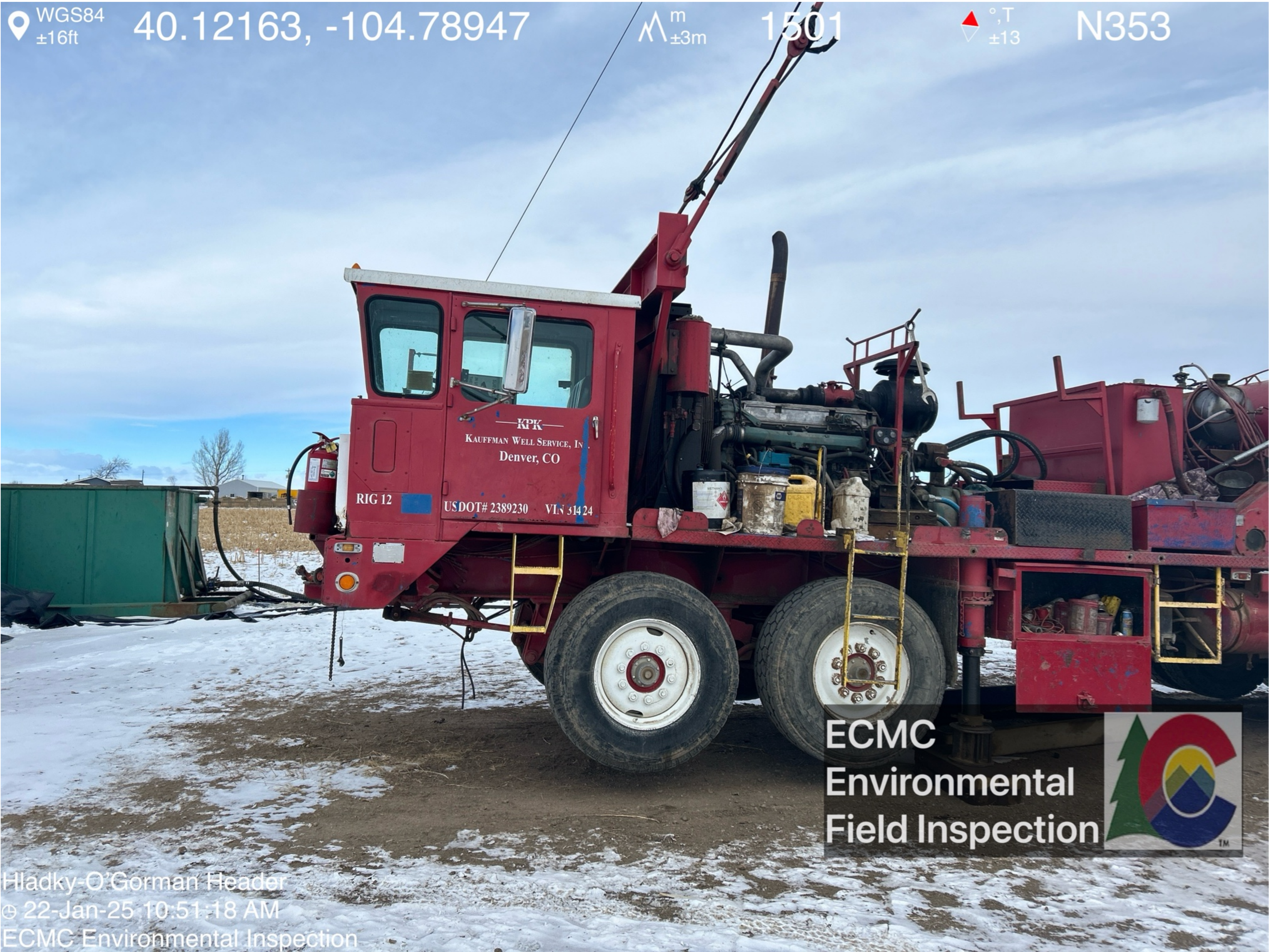
Operator rig on location for plugging and abandonment activities..
