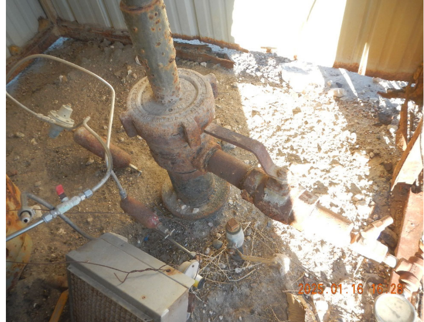
2. View of wellhead. Note debris on ground inside shed.
