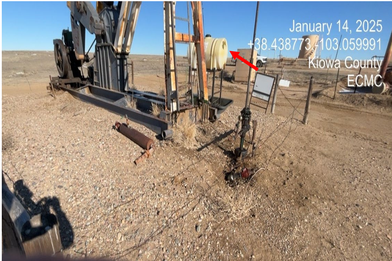
Photo 3. The plastic container at the pumpjack is broke and needs to be removed and disposed. Previous CA was not completed.
