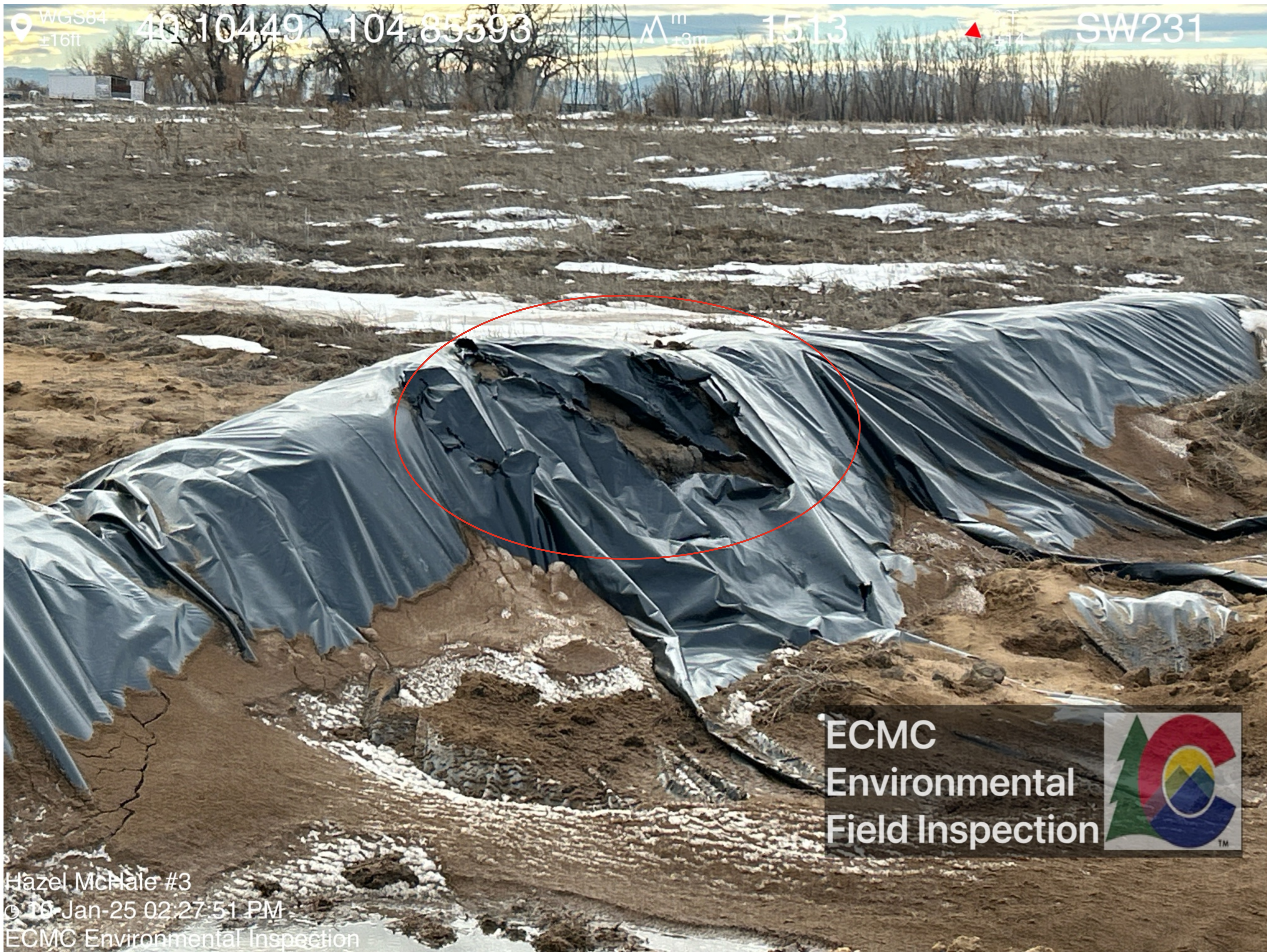
Holes/tears present in liner.
