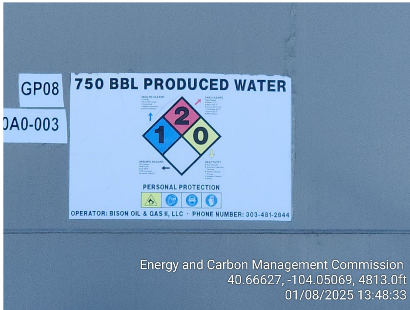
Photo 11 – 24 Hour Contact Name and Number not current
