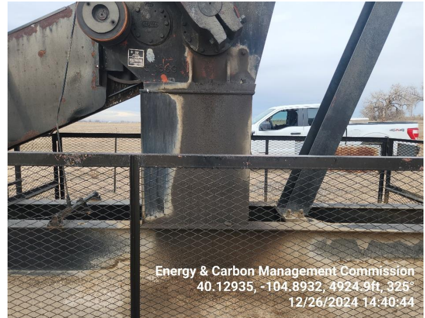
Photo 6 Leaking gasket staining pump jack concrete pad.
