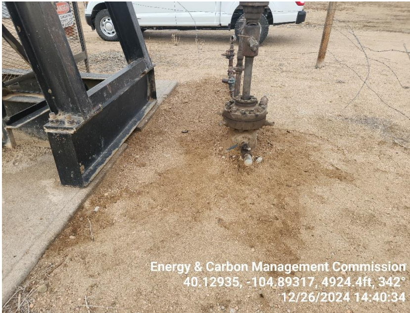
Photo 5 Stained soil around the wellhead.
