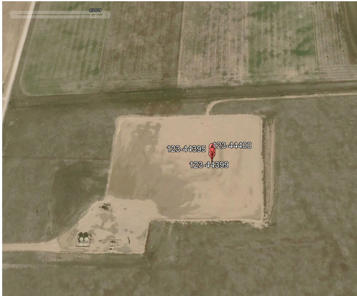
Photo 7. Google Earth aerial imagery (circa 09/2019) illustrating that location expansion for the drilling pad. AL wells 123-44395, 123-44400 and 123-44399 were not drilled based off of Form 4 Sundry notices indicating that the wells were not drilled and to abandon the permit. The location expansion/drilling pad appears to have been reclaimed at the time of this inspection, though the access road will need to be reclaimed
