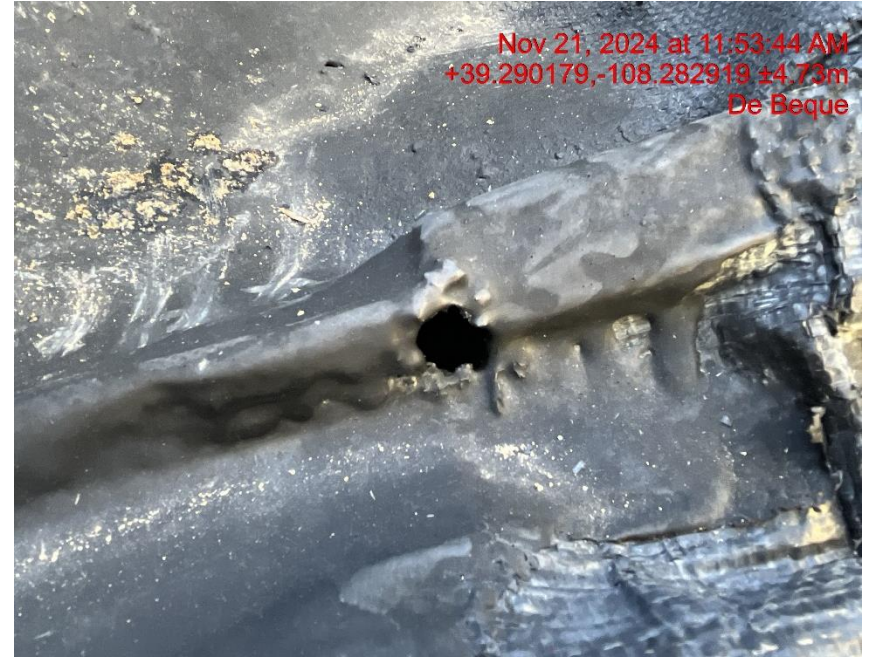
Photo # 9504 Multiple holes and tears in secondary containment liner/liner needs maintenance also the liner is deteriorating and lacks integrity
