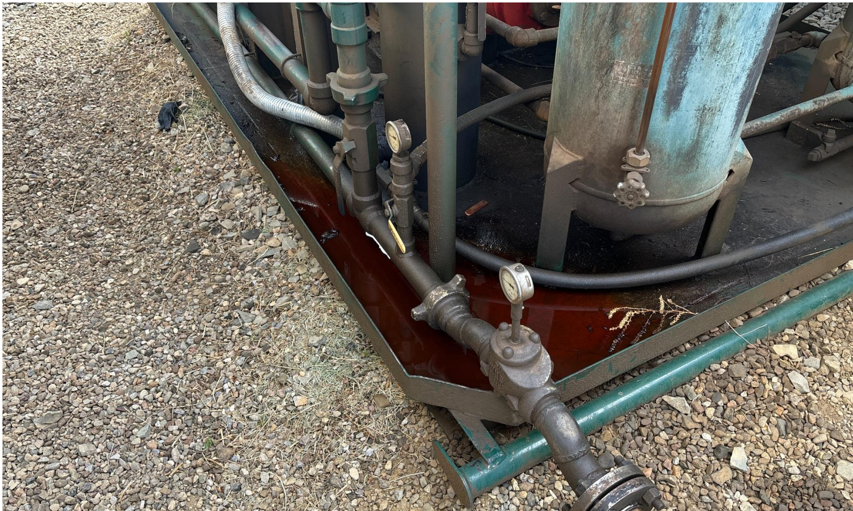
PHOTO 5: OILY WASTE FROM LEAK IN HYDRAULIC MOTOR HAS FILLED SKID AND HAS SPILLED OVER CAUSING IMPACT SOIL SURROUNDING SKID. DRAIN OILY WASTE REPAIR ALL LEAKS AND REMOVE OR TREAT IMPACTED SOIL PER RULE 1002..(2).D & 1002.f.(2)B, Comply with general provisions of the oil and gas act for wildlife protection AND SB-181. CA DATE 11/22/2024 TO DRAIN SKID 12/21/2024 DO REPAIR EQUIPMENT AND STOP LEAKS.
