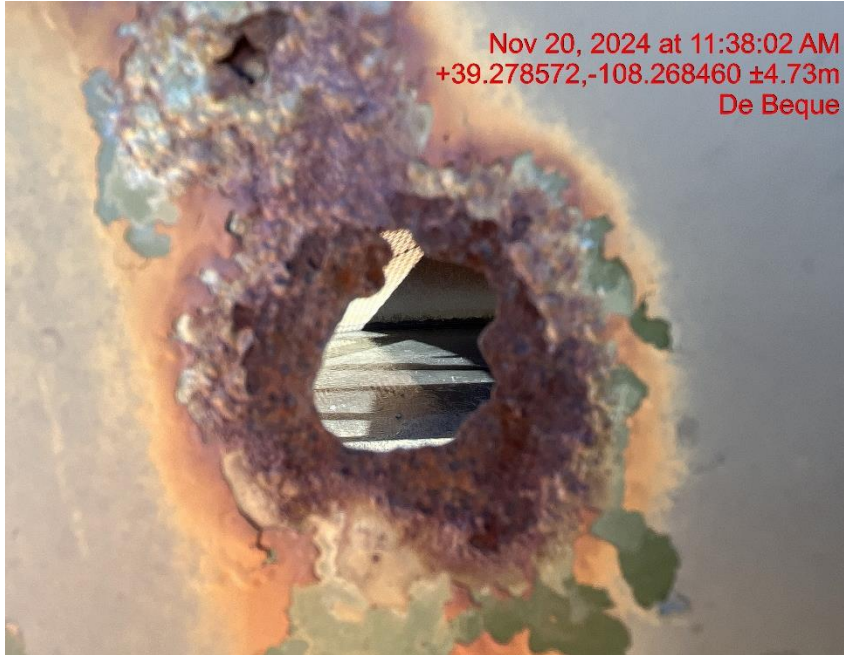
Photo # 9303 Tank failure/Tank lacks integrity
