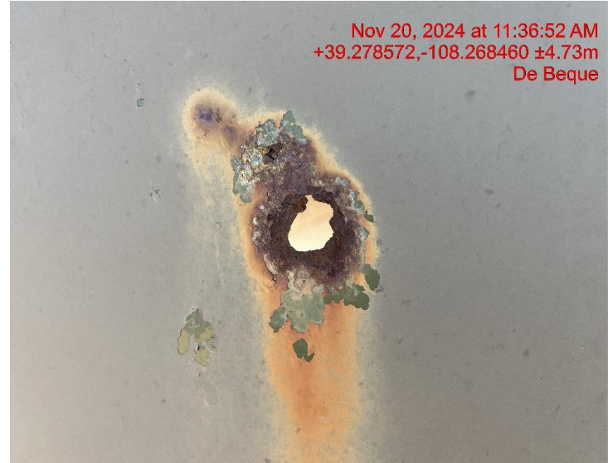
Photo # 9300 Tank failure/Tank lacks integrity
