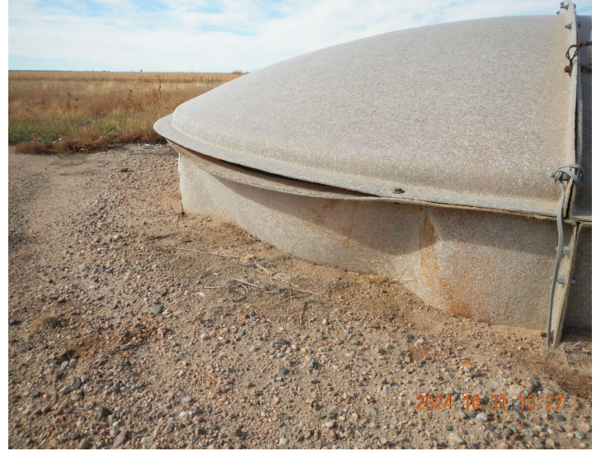
10. Additional view of separation on produced water tank.
