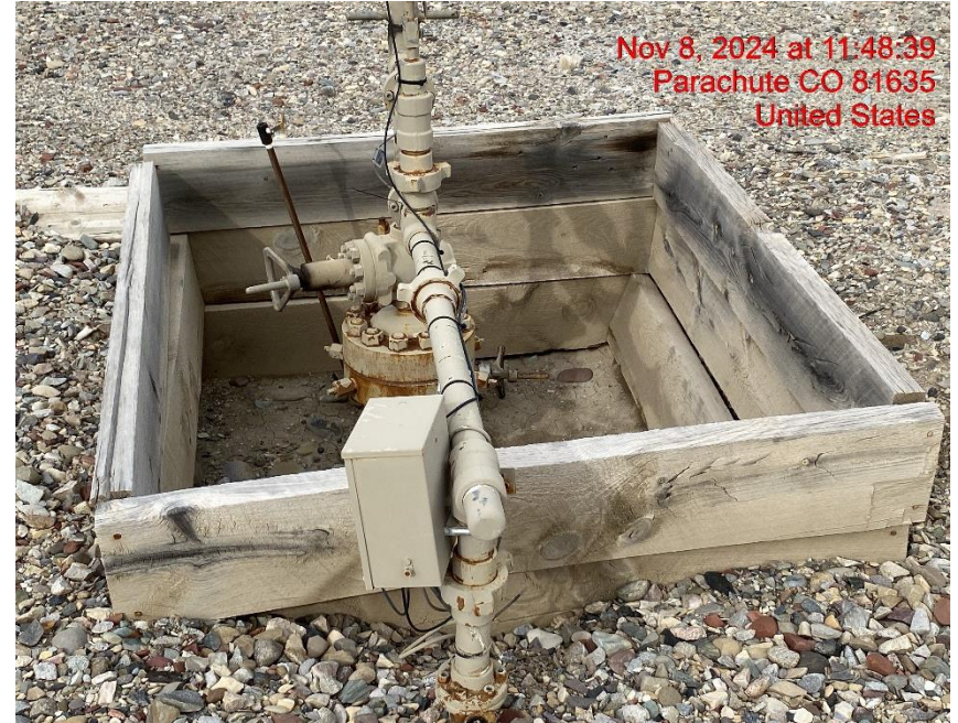
Open Wellhead Cellar/No Wildlife Egress – Photo #04804
