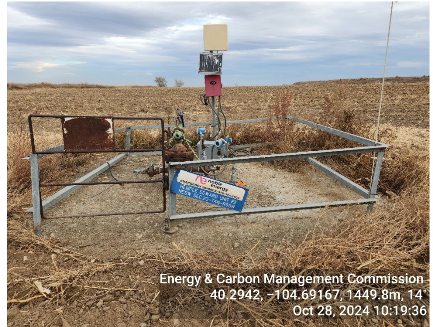
Photo 6: TA Wellhead
