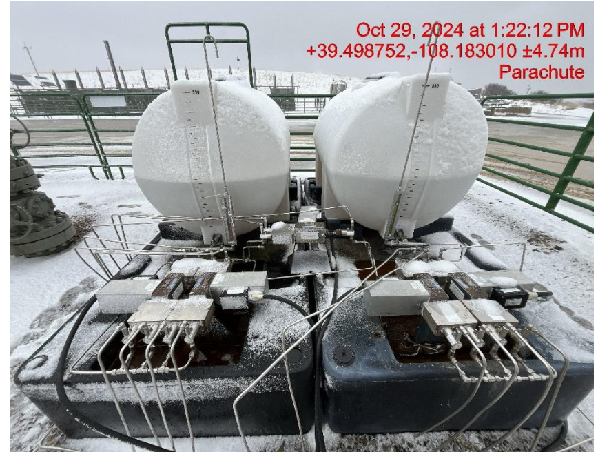
Photo # 8217 Failure to maintain chemical BMP's/chemical containments full of fluid & not sufficient to contain possible spill
