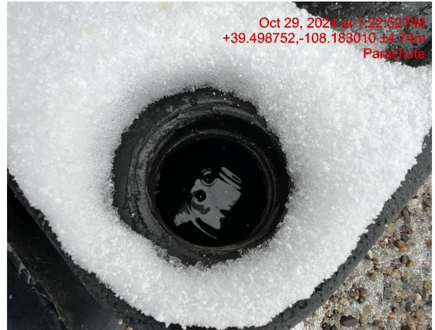
Photo # 8221 Failure to maintain chemical BMP's/chemical containments full of fluid & not sufficient to contain possible spill
