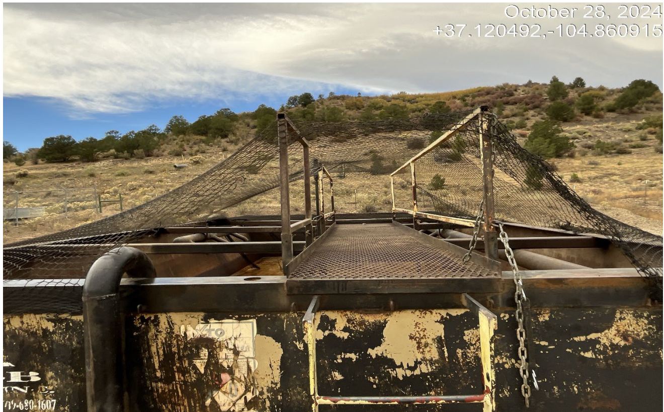
Photo 6. The netting on the open top tank does not cover the entire open top tank. Previous CA was not completed.
