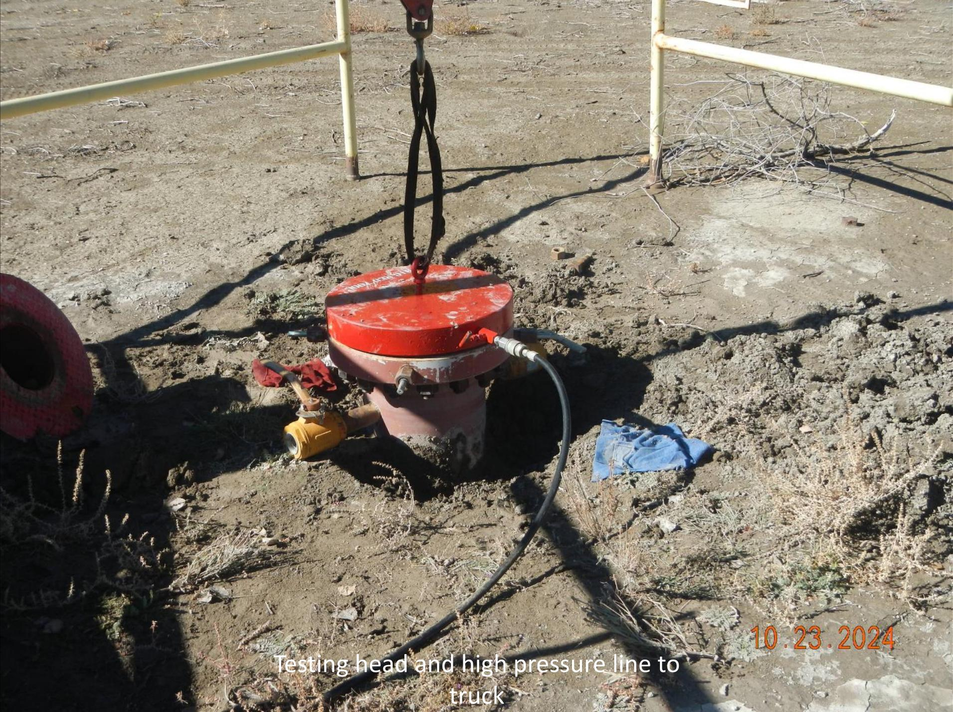
Testing head and high pressure line to truck
