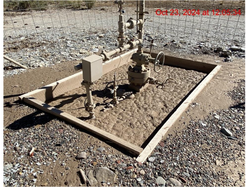
Open Wellhead Cellar/No Wildlife Egress – Photo #04429
