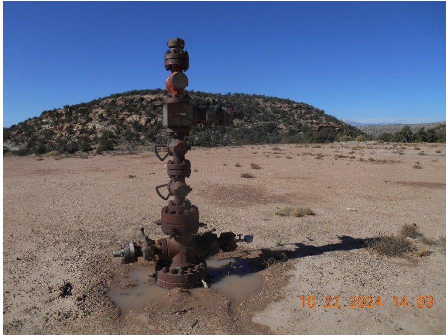
Wellhead – Temporarily Abandoned
