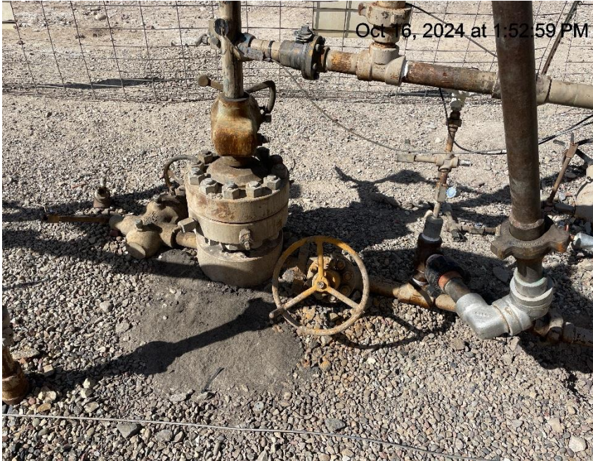
Photo # 6139 Staining near wellhead
