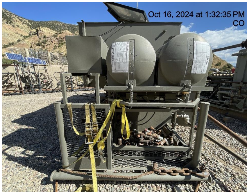
Photo # 6140 Chemical tanks lack BMP's
