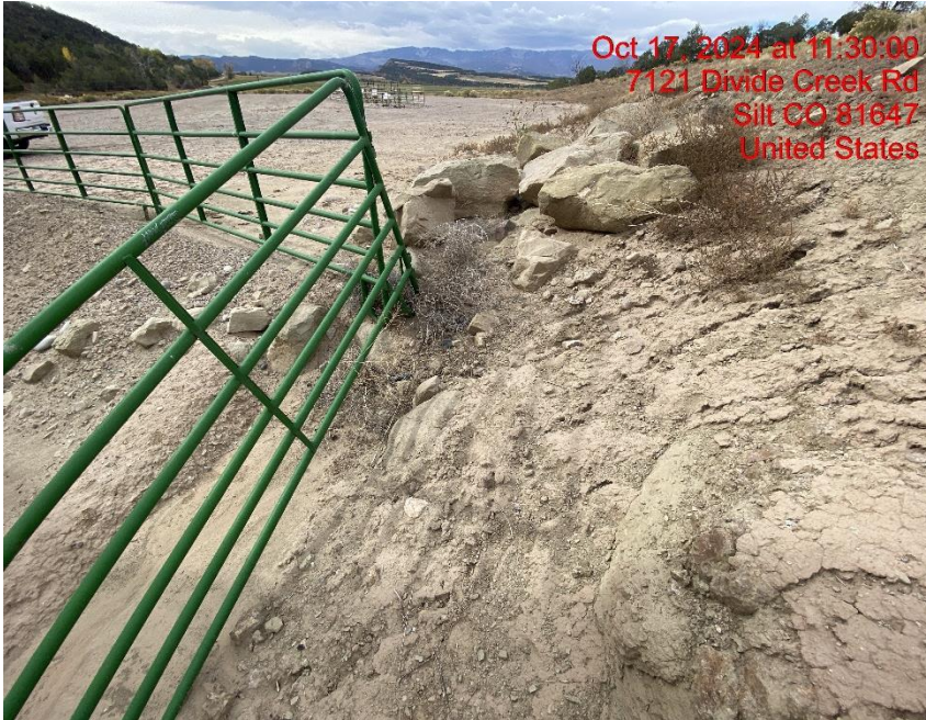
Insufficient Erosion Control/Degradation – Photo #04279
