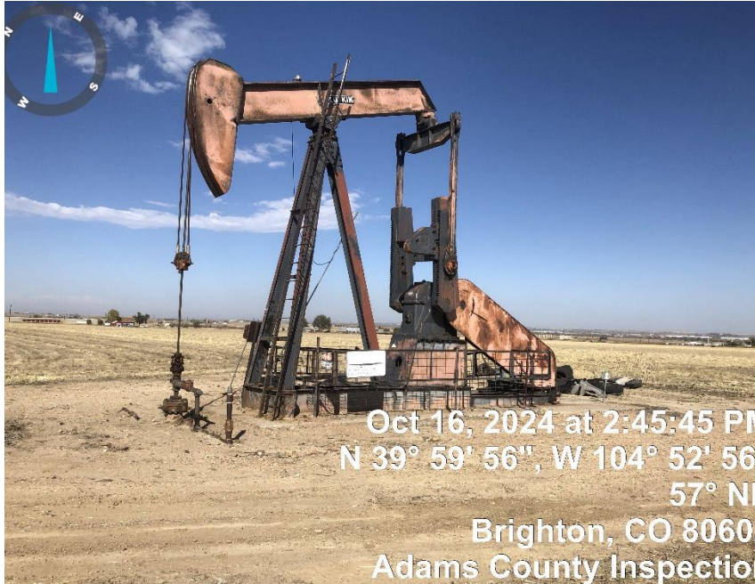
Photo#1 Pumpjack/Wellhead
