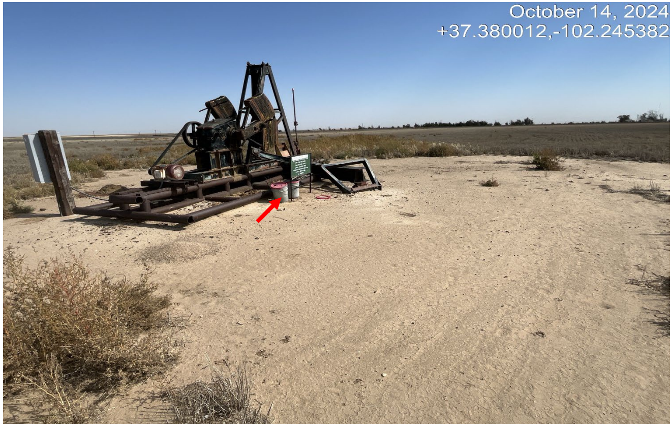
Photo 5. There is buckets of chemical at red arrow that need to be removed.
