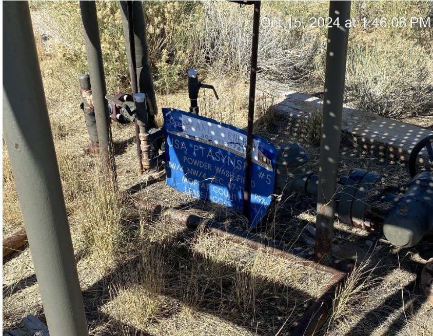
Well sign on the ground and missing required information
