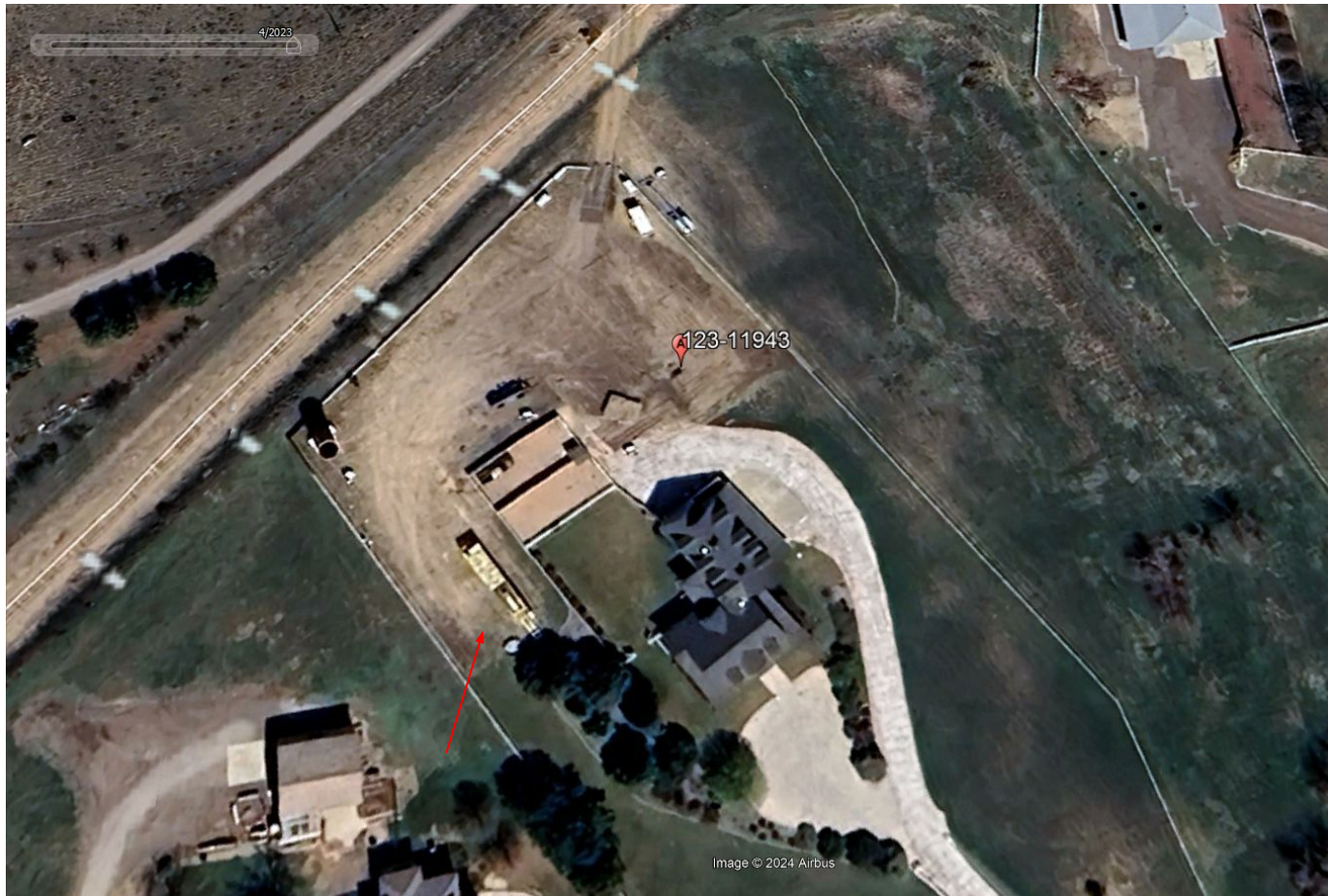
Photo 11. Google Earth aerial imagery (circa 04/2023) illustrating that equipment appears to have been staged on the southern/southwestern portion of the disturbance area (in reference to Photos 7-10); these areas could potentially be compacted and/or were not reclaimed.
