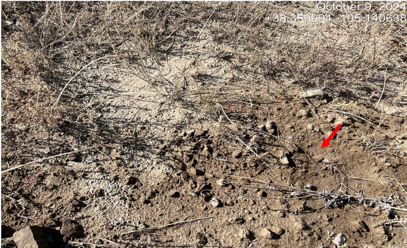
Photo 6. Discolored soils shown in previous photo have a diesel fuel odor. This must be cleaned up.
