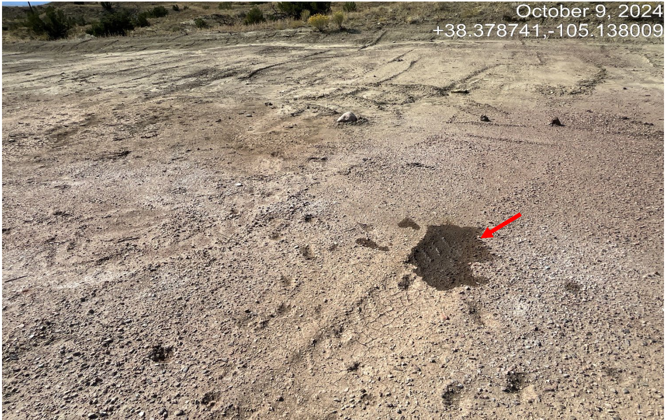
Photo 6. There was previous impacts observed and there is oil stained soil shown at red arrow. The area of the tank battery and abandoned well need to be sample per form 27 decommissioning of the well.
