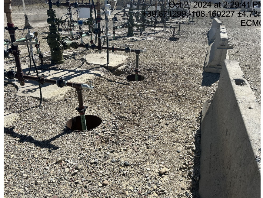
Open holes at well heads
