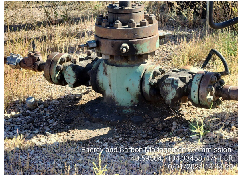
Photo 4 – Wellhead – Stained Soil
