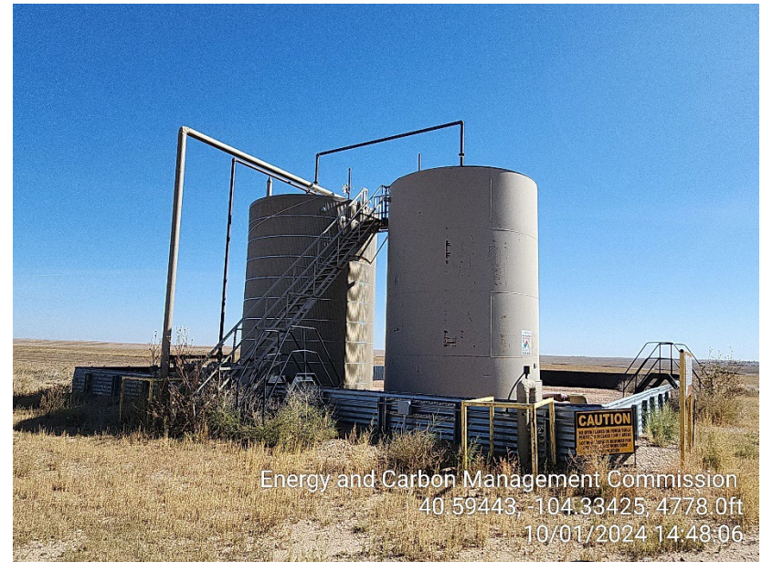
Photo 12 – Tank Battery
