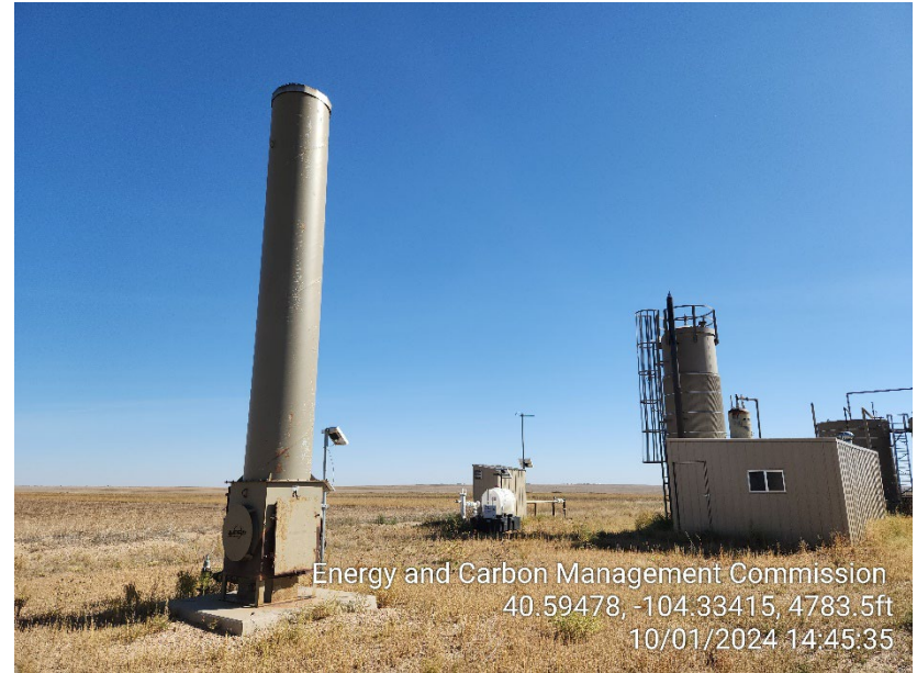
Photo 6 – ECD and Heater Treater
