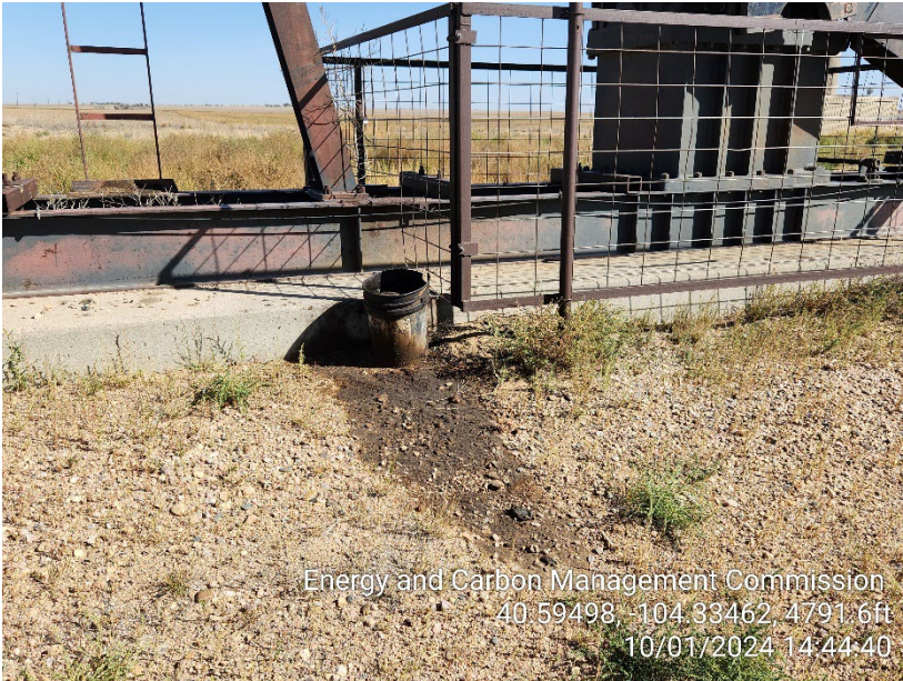
Photo 5 – Oily Waste and Stained Soil at Pumping Unit
