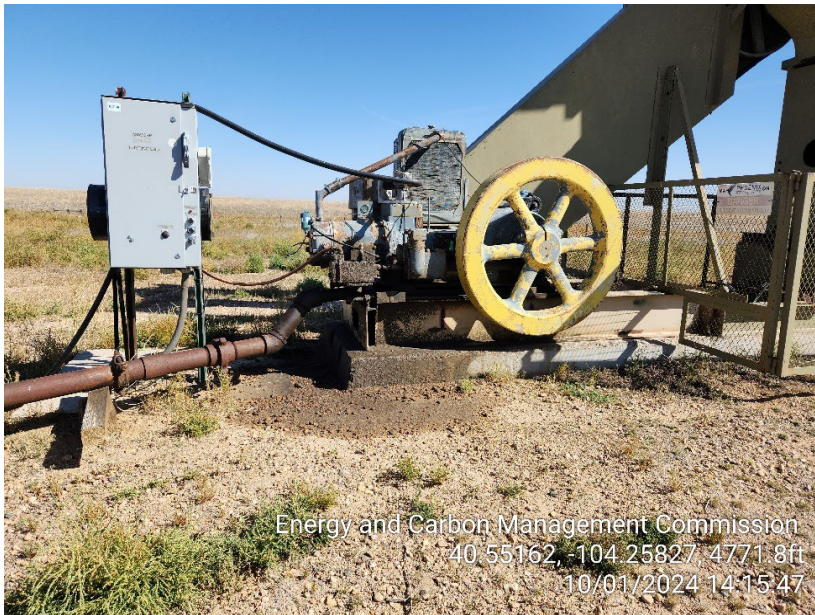
Photo 3 – Stained Soil at Gas Engine
