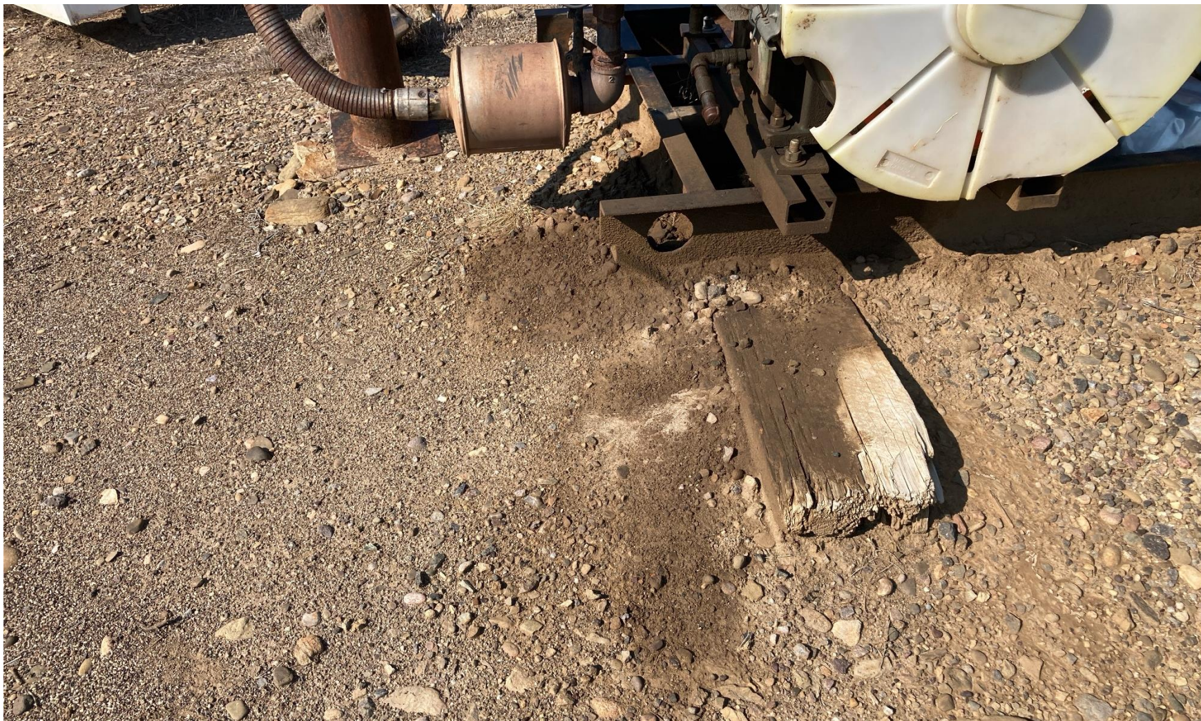
PHOTO 4: AREA OF IMPACTED SOIL AROUND THE DEER 23-17 PUMPJACK PRIME MOVER. Conduct maintenance on equipment, cleanup stained material and review self inspection processes. COMPLY WITH RULE 1002,.(2).D CA DATE 11/08/2024.
