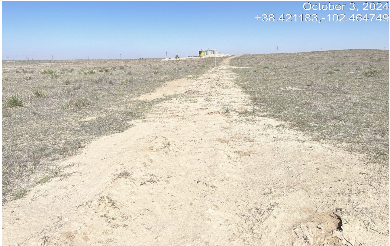
Photo 1. Facing north along the flowline disturbance. The soils along the flowline need to be regraded and reclaimed.
