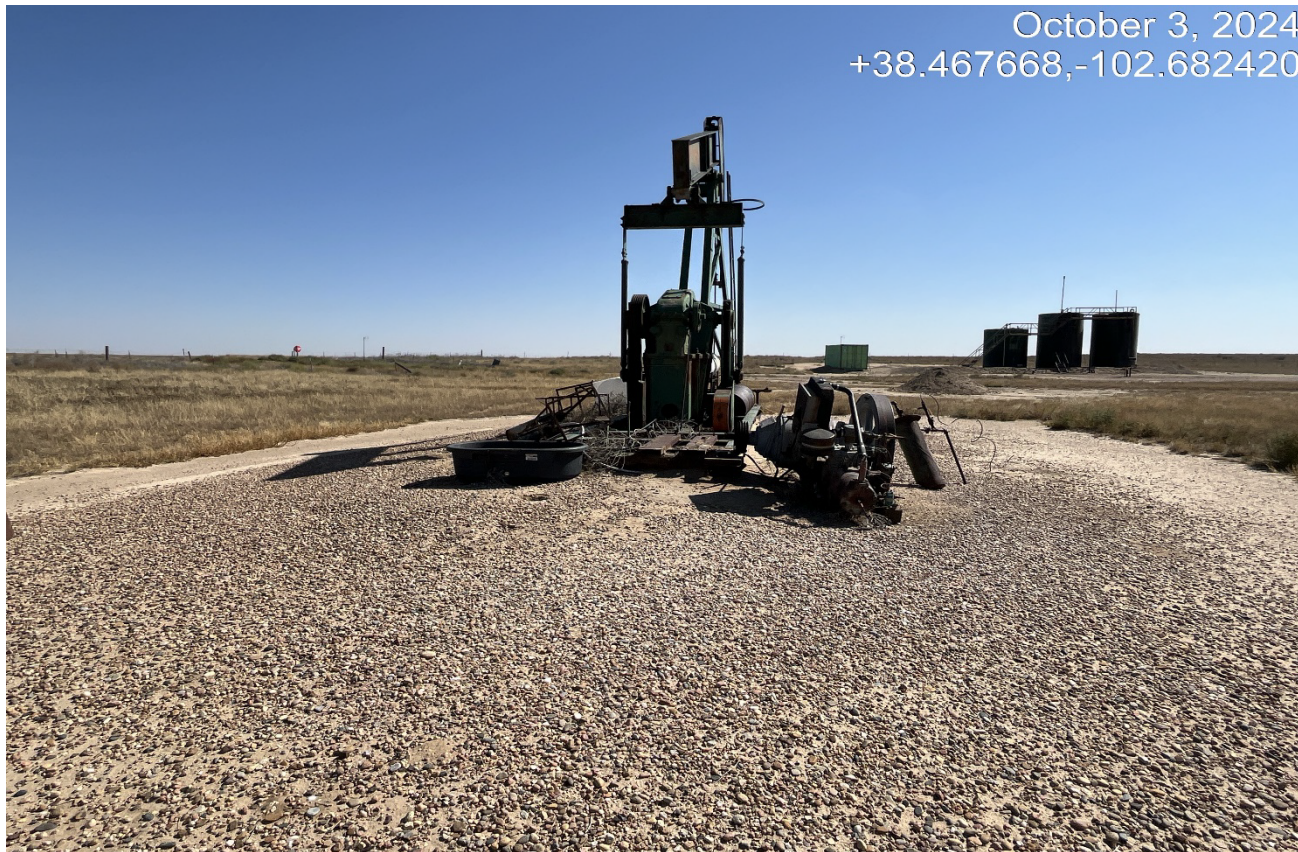
Photo 9. The chemical container at the backside has also tipped over. There are unused parts of the pumpjack laying on the ground that need to be removed.
