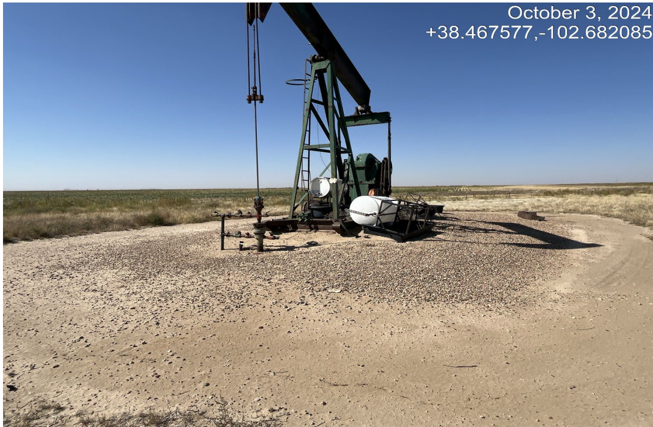
Photo 8. Facing toward the wellsite. The chemical container has tipped over. Previous CA was not completed.
