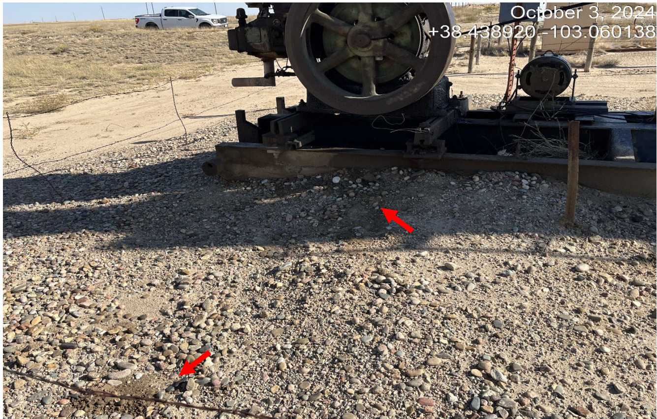
Photo 6. There is still oil stained soils at the back side of the pumpjack that must be cleaned up. Previous CA was not completed.
