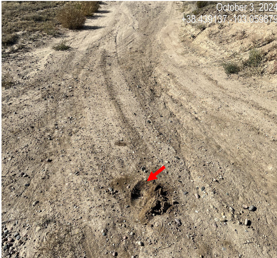
Photo 3. View of the stained soils that still remains along the road where oily material was spread along the road.
