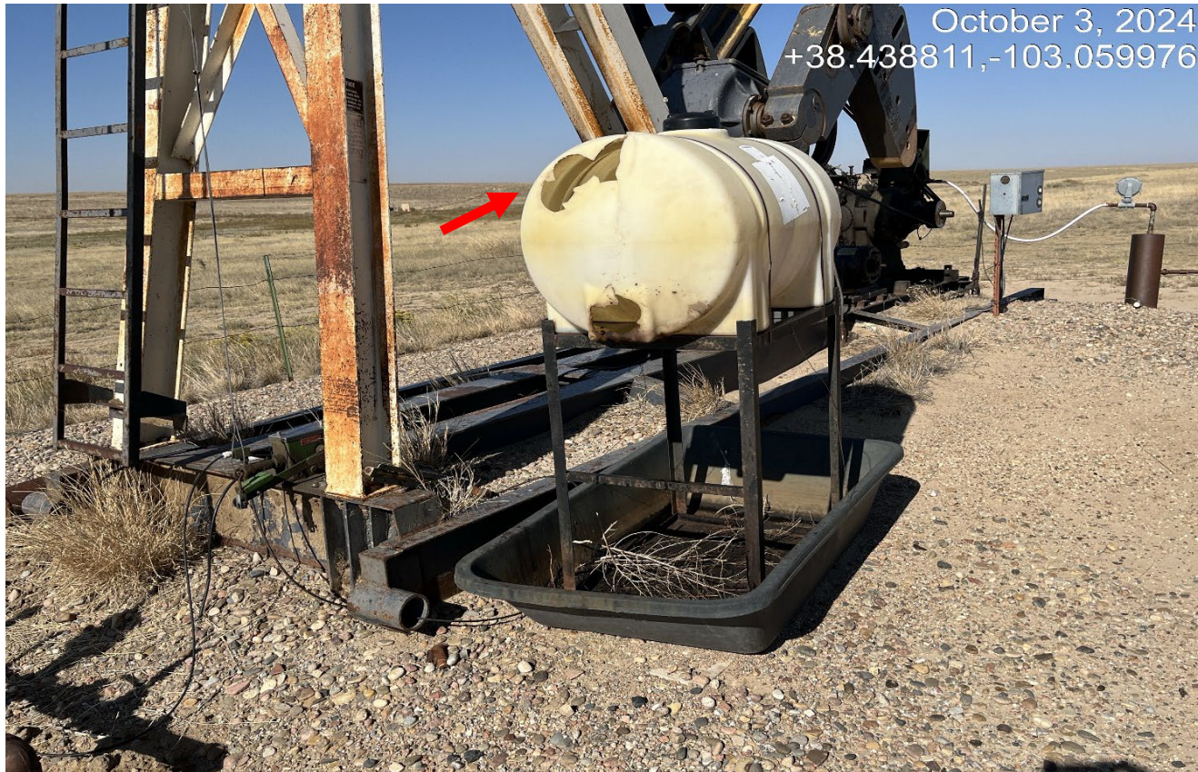
Photo 7. The plastic container at the pumpjack is broke and needs to be removed and disposed.
