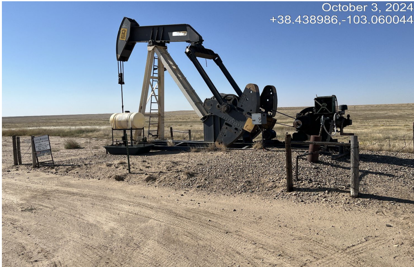
Photo 5. Facing toward the pump jack. A new well sign has been installed. The 2 wire fence around the equipment is not sufficient to prevent livestock entry.
