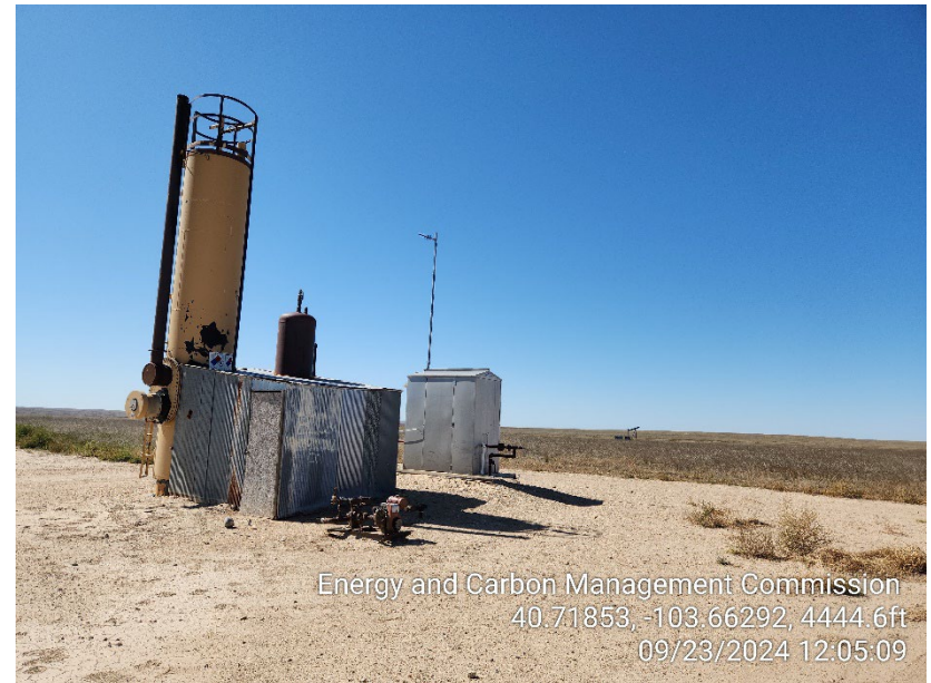
Photo 8 – Heater Treater and Gas Meter
