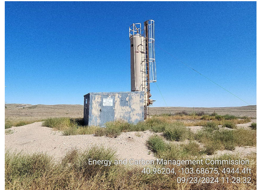
Photo 4 – Heater Treater
