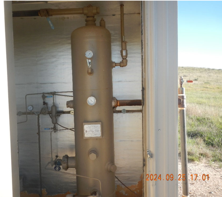
4. Vertical separator inside separator shed.
