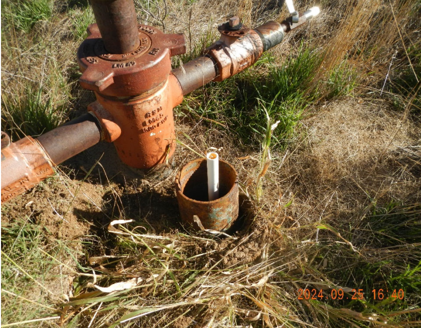
3. View of possible Bradenhead piping with no valve or fittings.
